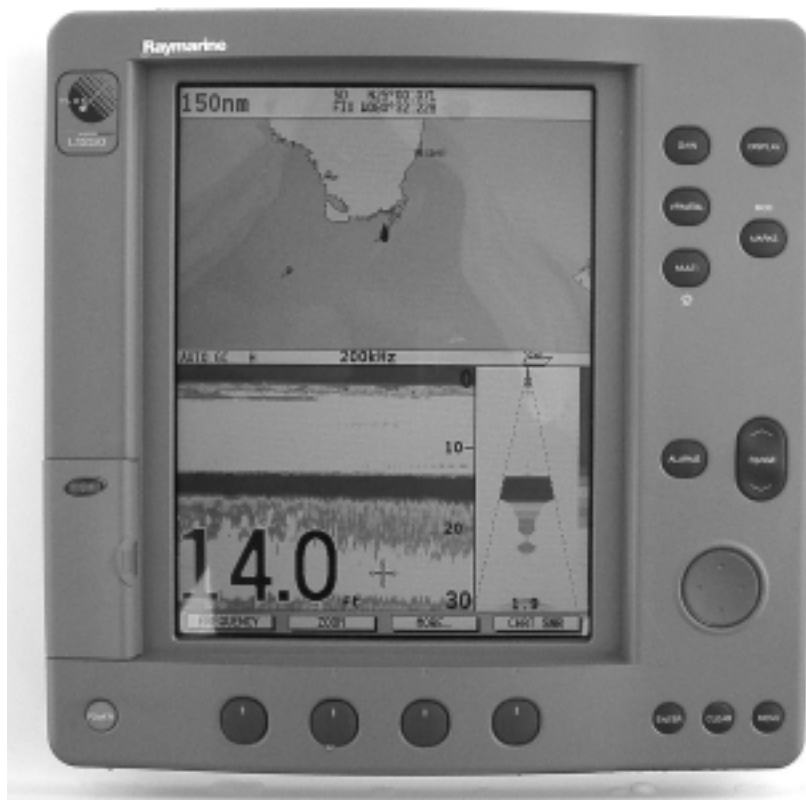
Above: The screen of the Raymarine HSB 2 is split horizontally to create two displays. Here, a chart is pictured on top, with a depth sounder screen on the bottom. The Furuno machine can do the same, and then actually split one of the smaller screens so three pictures are shown.
